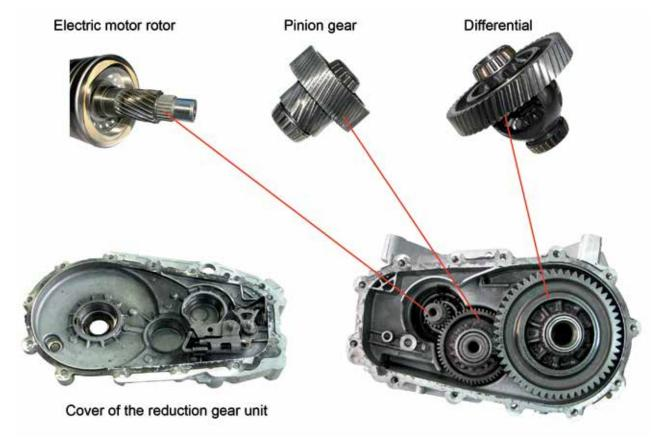
For the reverse operation, the coupling of a third pinion is also not required, as it is enough to reverse the rotation of the electric motor.
