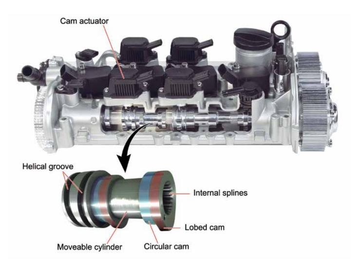
The cam cylinder is fixed in a specific position by means of a spring and ball retainer and its axial displacement is achieved by the action of one of the two deactivation actuator rods (cam actuator) on a helical groove machined into the cam cylinder itself.
