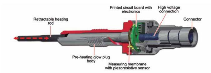
After filtering, the information obtained from this sensor is transmitted to the engine control unit, which then adapts the injection flow and advance throughout the engine rpm range. This optimises the combustion process to prevent the formation of **particulates and nitrogen oxides**
