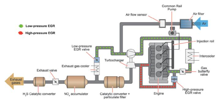
In short, this complex exhaust gas recirculation system reduces nitrogen oxides (NOx) to a great extent as it quantitatively reduces the amount of air (N2 + O2) taken in by the engine.
