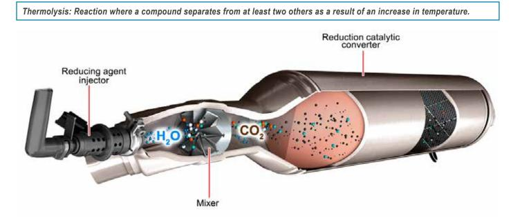
Next, the isocyanic acid undergoes thermal decomposition when it reacts with water. At the end of the hydrolytic section, the reducing agent decomposes and forms carbon dioxide and ammonia. Am-
